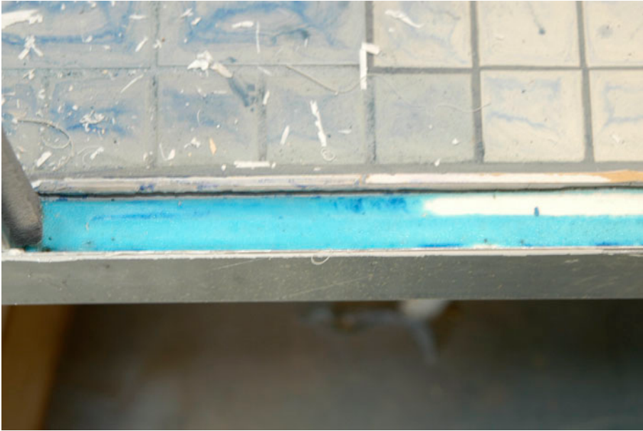
Figure 2. Groove along edge of floor element acting as substrate for wall elements.
