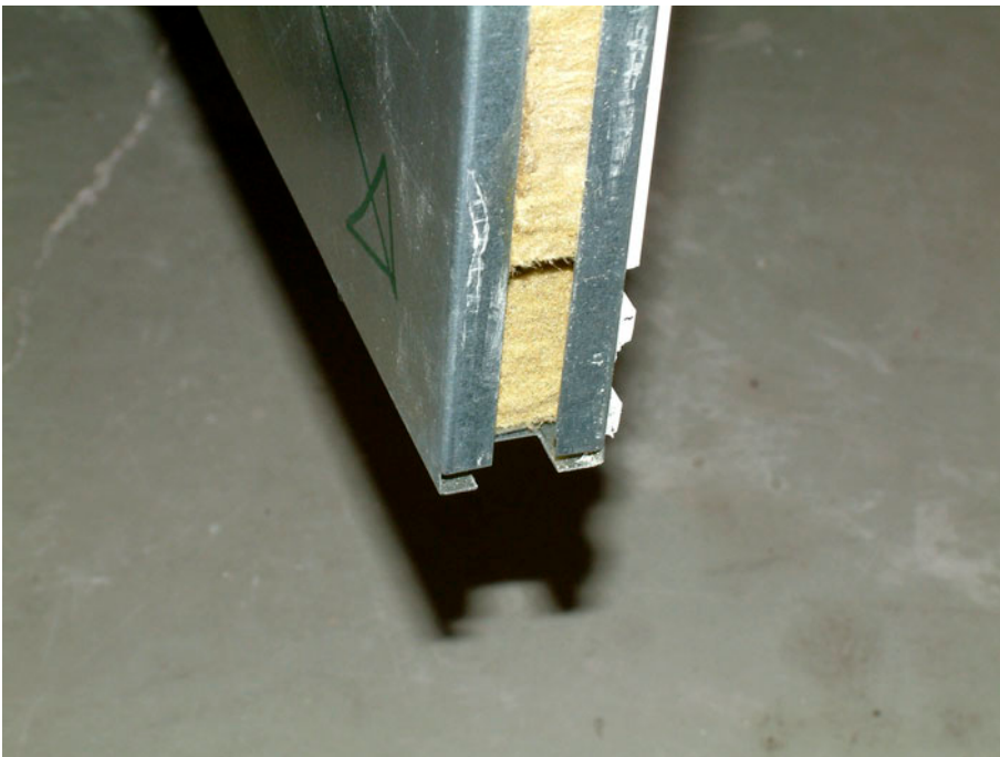
Figure 3. Corner of wall element after impact against floor.
